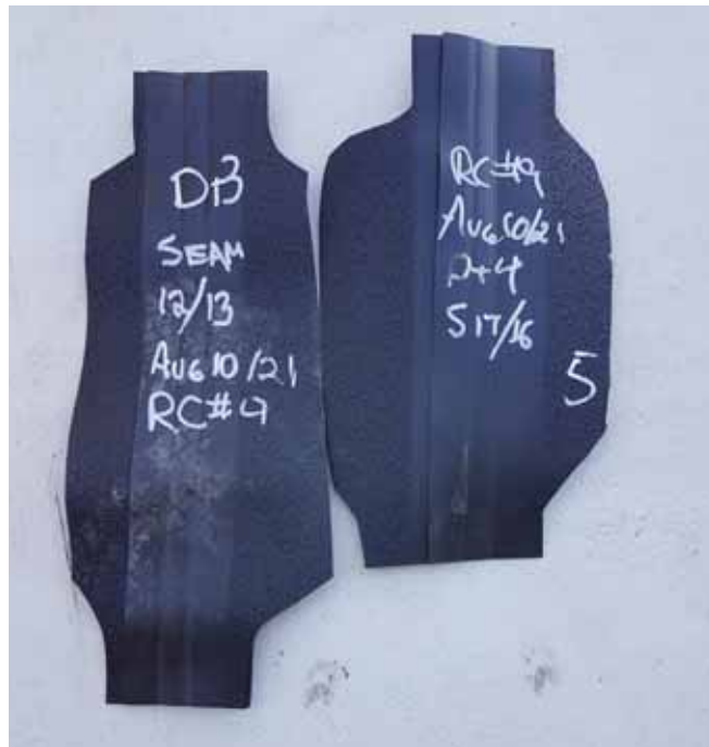
Photo 10 Typical Destructive Samples of Geomembrane Seams for Lab Testing
