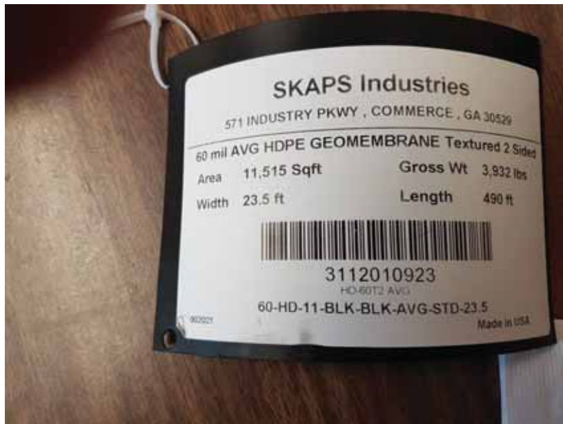
Photo 8 Typical Geomembrane Tag
